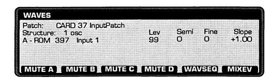
If your source is stereo, change the structure to 2 osc structure. Assign Input 1 as wave A and Input 2 as wave C, and then go to the PATCH BUS ASSIGNMENT page. Set Wave A ON for only Bus A, and Wave C ON for only Bus B, as shown below. This will cause the inputs to be hard-panned, left and right, to the stereo outputs. Make sure that the FX Bus parameter on the Performance Part Detail page is set to PATCH, so that the assignments you just made will be used.
