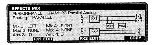
If you're using only the stereo outputs (1 and 2), you should go to the Effects Mix page and set Mix 3 and 4 to Left and Right, respectively. This will ensure that the output of Effect 2 is included in the mix. Setting the Mix 3/4 parameters to OFF will remove them from the stereo mix, sending them to outputs 3 and 4 only. For more information on the Effects Mix page, see Section 7.2, Effects Buses and Routing.
