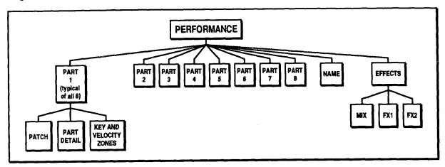
Performances consist of eight Parts. Each Part is a Patch together with some adjusting parameters (PERFORMANCE PART DETAILS) and a playback range (KEY AND VELOCITY ZONES).
