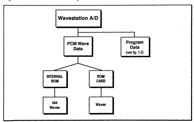
Figure 1-3 Wavestation A/D Memory Banks - PCM Wave Data
