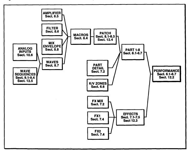
Figure 6-1 Wavestation A/D Performance Signal Flow
