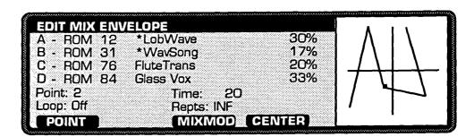
If the Patch is in 2 oscillator mode, the B-D axis (Y-AXIS) disappears. Waves A and C continue to be affected by the Mix Envelope.
