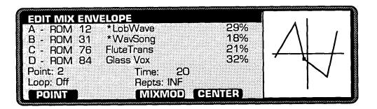
To set the levels of the mixer envelope, select a point and then use the joystick to set the position.
