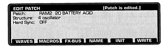
The Patch selected here is the Patch in the Part highlighted on the Edit Performance page. Likewise, changing the Patch selected on this screen changes the Patch in the highlighted Part.
