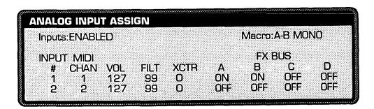
For sending a monophonic source through Effect 2 only, you can use the C-D MONO Macro, adjusting the Effects Mix accordingly.
