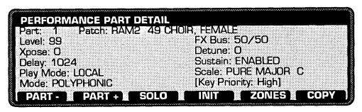
This page shows the details of each Performance Part. At the top of the page is the most important parameter: the name of the Patch assigned to this Part.
