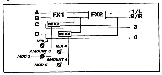
Input at A/B goes through FX1 and FX2 to output 1/2. Inputs C/D are left unprocessed at the outputs 3/4, or can be dynamically mixed (wet/dry) into FX2 as well.
