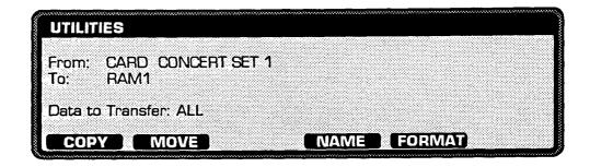
This page lets you quickly transfer complete sets of Performances, Patches, and Wave Sequences between cards and internal memory. (For transferring individual Performances and Patches, use WRITE.)
