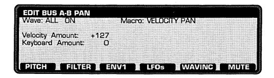
This page sets the modulation of the Pan position, the left-right orientation of the sound within the stereo field. Pan may be modulated by velocity and keyboard position (MIDI note number).
