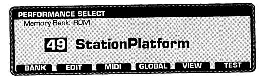
The PERFORMANCE SELECT page is the highest level of the Wavestation A/D's menu system. It appears when you switch power on or after you press the EXIT switch a sufficient number of times.
