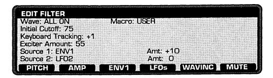
The filter module determines overall tone color. The FILTER page contains the frequently-used Cutoff and modulation Source settings. In practice, you often need to balance these adjustments against each other.
