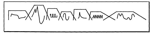
Note that this rough drawing is not a waveform, but a picture of the overall amplitude envelope of the wave sequence. Generally, a Wave Sequence crossfades between the wave steps.
