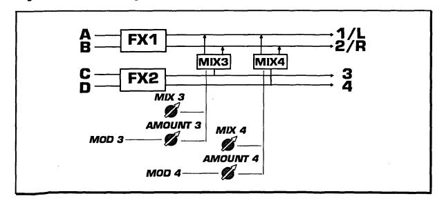
In Parallel routing, the panned input at A/B goes through FX1 to output 1/2. Input C/D goes through FX2 to output 3/4. Also, FX2 can be mixed into the 1/2 output through MIX3 and MIX4. This gives you dynamic control over the panning.
