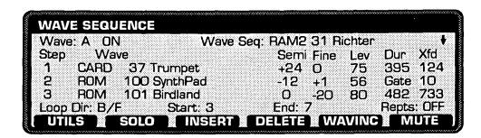
Here is where you select the waves for each step of the selected Wave Sequence. Loop control is also included on this page.
