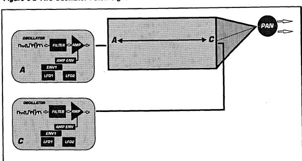
Figure 8-2 Two-Oscillator Patch Signal Flow
