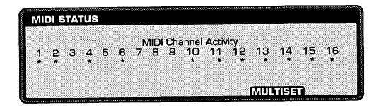
The Wavestation A/D includes a feature that is very handy when you are troubleshooting your MIDI setup. The STATUS page shows graphically when and on what channel data is being received at the MIDI IN jack. When data is received on a particular channel, the asterisk (\*) under its number appears. If data is not being received, you know that the problem probably lies in either the MIDI controller or, more likely, a cable or its routing.
