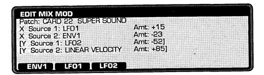
Each of the two mixer dimensions can have two modulating sources in addition to the mixer envelope (and joystick).
