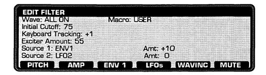
The classic 24 db/octave low-pass filter sets the basic Patch timbre or shapes it over time in response to physical or programmed controllers.
