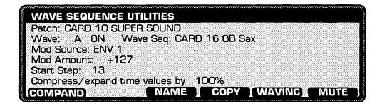
This page allows you to modulate the starting step of the Wave Sequence, or to use a mod source to control the progression from step to step. It also lets you stretch or shrink the overall time of a Wave Sequence.
