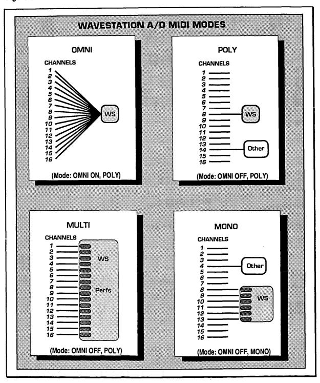
**NOTE:** In MULTI and MONO modes, local and incoming MIDI controllers are kept separate, so that the sound will not be affected by moving the local joystick unless it is being routed back to the Wavestation A/D via MIDI. In OMNI and POLY modes, local and MIDI controllers are shared.
