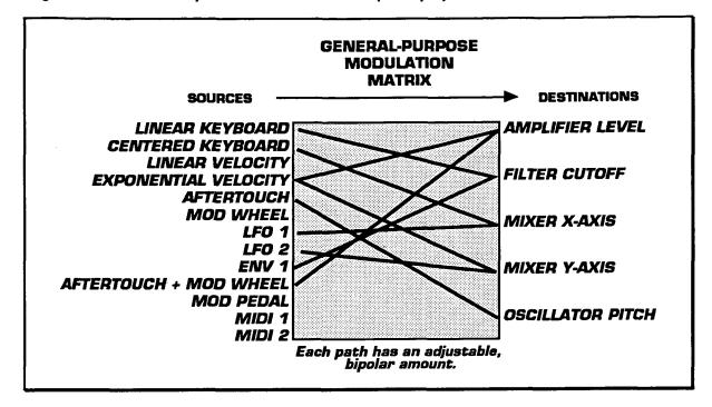
Figure 8-5 General-Purpose Modulation Matrix (example)
