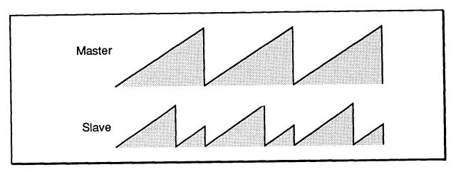
Since the overall timbre depends upon the pitch relationship between the slaves and the master oscillator, you can vary the timbre by modulating the pitch of the slaves. The pitch shift can be subtle (usually by LFO) or extreme (usually by envelope), as in the case of the classic "swept-sync" patch.
