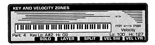
The KEY AND VELOCITY ZONES page graphically displays the keyboard layers and splits, as well as velocity ranges programmed into the Performance. In general, Patches create sound and can be thought of as instruments, while the Zones and Details determine how the eight instruments play together.
