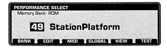
The large current Performance number and name actually displayed on your instrument may be different from this example. When you power up the Wavestation A/D, it will remember the Performance that you had selected before last turning it off.
