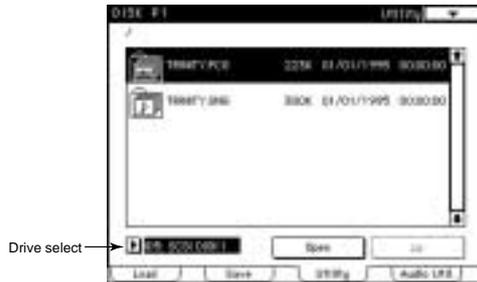
When using Drive Select to select a hard disk, the ID numbers of hard disks that have not been formatted will appear as Unformatted, and the ID numbers of hard disks that are not connected will appear as None. Even if a hard disk has been formatted by a personal computer, etc., it will be shown as Unformatted, and such a hard disk must be formatted as well.
