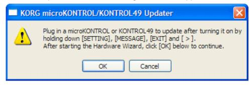
4. Hold down the [SETTING], [MESSAGE], [EXIT], and [OCTAVE SHIFT / CURSOR >] keys, and then turn on the power of the microKONTROL / KONTROL49. (Note: Nothing will appear on the microKONTROL / KONTROL49 display - don't worry!) The microKONTROL / KONTROL49 will be recognized as a new device, and the following "Found New Hardware Wizard" window will appear. After this, press the [OK] button in the window that appeared from step 3 above.
