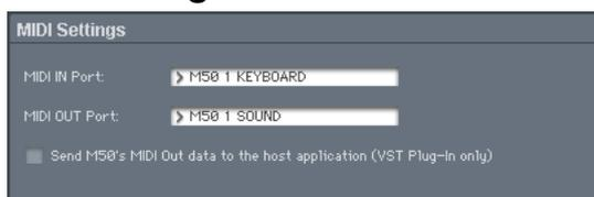
Here you can adjust settings for MIDI connections between the M50 Editor and the M50.
