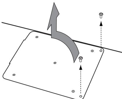
2. Make sure that the EXB-RADIAS is oriented correctly, and use the five screws to fasten it to the back of cover "A."
