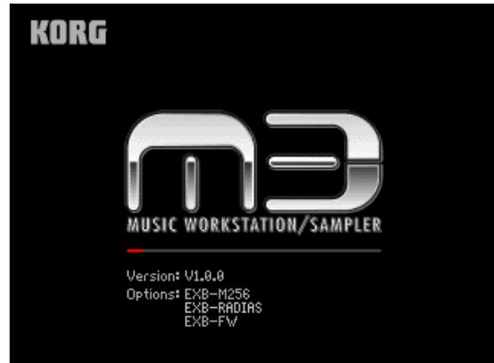
After installing memory or an option board, you must turn on the power and verify that the name of the item you installed is shown in the display.
