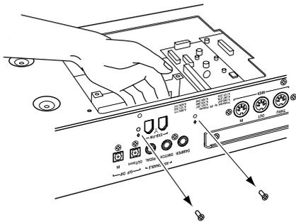
3. Verify the location in which you'll be installing the EXB-FW, and align it so that the connector section of the EXB-FW protrudes from the rear panel of the sound module.
