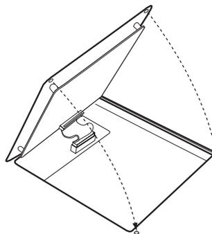
5. Fasten cover "A" using the two screws you removed in step 1.
