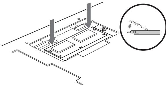
4. Attach cover "B" to the sound module, and fasten it using the two screws you removed in step (2).
