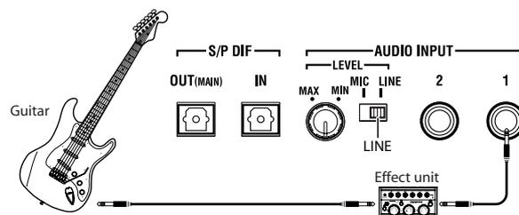
**!** If you connect a guitar with passive pickups (i.e., a guitar that does not contain a preamp), you will be unable to sample it at the correct level because of the impedance mismatch. Such guitars should be routed through a preamp or an effect unit.
