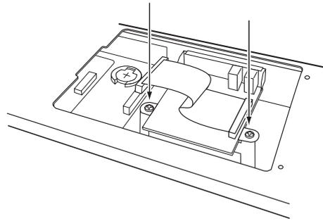
5. Tighten the two screws you removed in step (2) to fasten the EXB-FW to the rear panel of the sound module.
