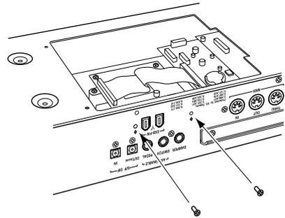
6. Attach the cable as shown in the illustration. Firmly insert the cable as far as it will go.
