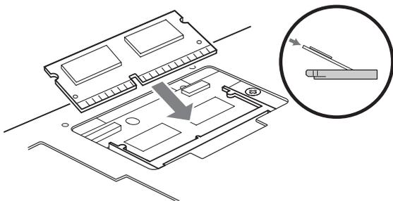
3. As shown in the illustration, gently press down the EXB-M256 so that it lies flat. When the EXB-M256 clicks into place, locking tabs will hold it in place.
