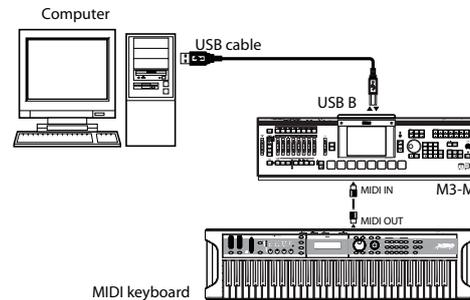
If you're using the M3 Plug-In Editor or a DAW, you can connect your MIDI keyboard via your computer as shown in the following illustration, instead of using the connections shown in the illustration above. (If you connect to your computer via MIDI, you'll need a commercially available MIDI interface.)
