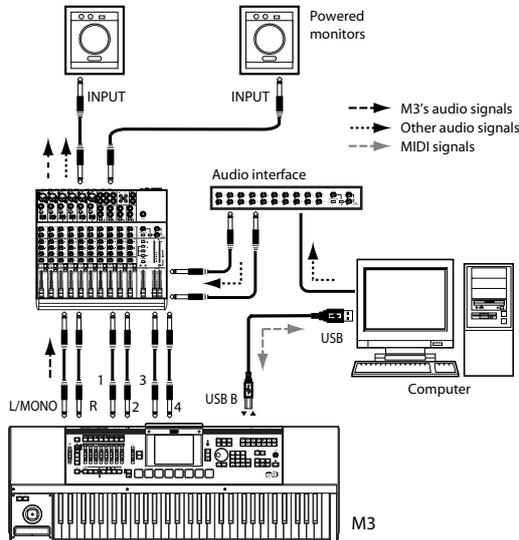
If you want to apply a plug-in effect to the M3's audio signals, or to control the M3's audio signals in your host application together with the audio data from the KORG Legacy Collection or other audio tracks, make connections as shown below. Make settings as appropriate for the host application you're using.
