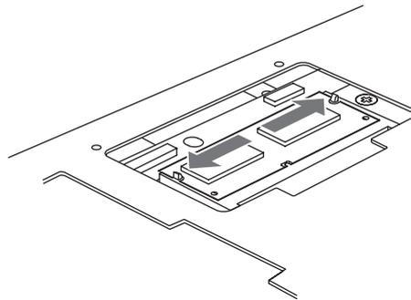
3. Pull the EXB-M256 straight out and remove it from the slot.
