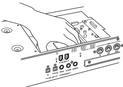
4. Tighten the two screws attached to the EXB-FW to firmly fasten it to the sound module.
