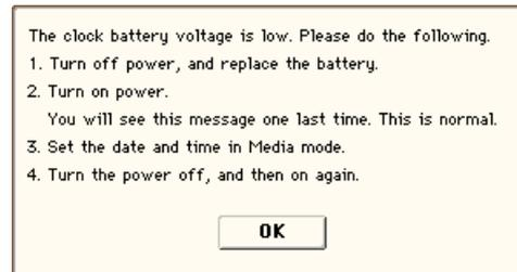
Make sure that you are not using a battery that has run down, and that the battery is installed correctly.
