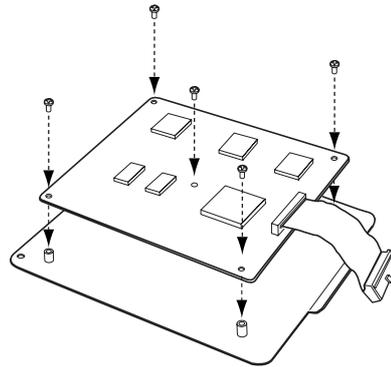
3. Connect the cable of the EXB-RADIAS to the connector of the sound module as shown below.
