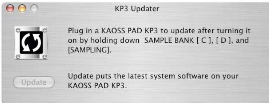
3. Hold down the SAMPLE BANK [C], [D], and [SAMPLING] buttons, and then turn on the power of the KAOS PAD. (The display of the KAOS PAD will indicate “IPL”.)
