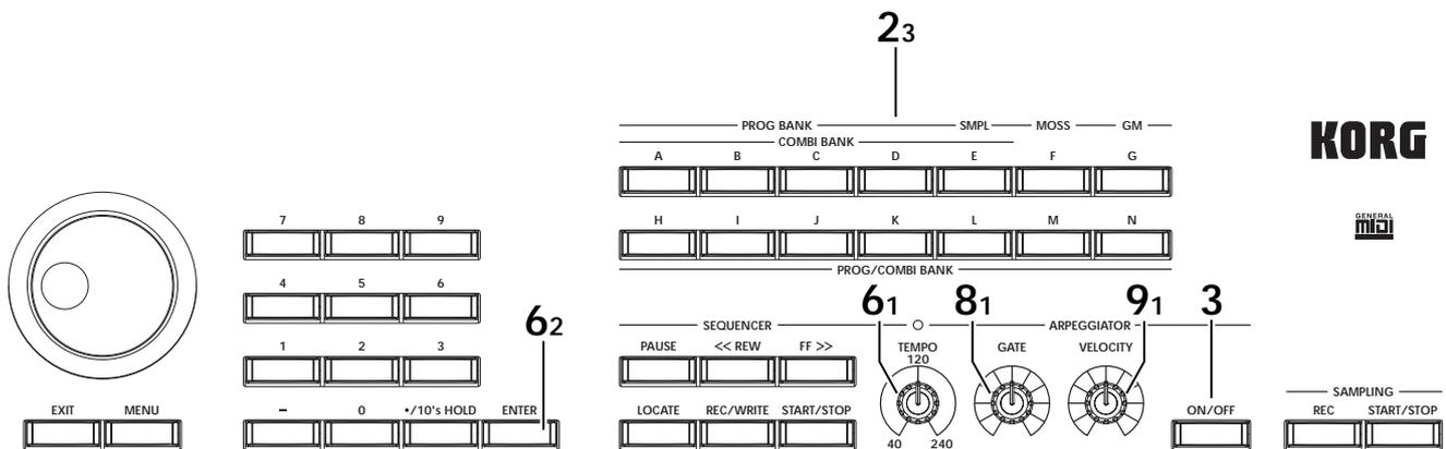
**note** Another way to set the tempo is by selecting “♩=” and using the [△][▽] keys or the [VALUE] slider. You can also synchronize the tempo to an external MIDI device. In this case you won’t be able to control the tempo from the TRITON Extreme. The apparent tempo is also affected by the “Resolution” setting in the P7: Edit-Arpeggiator, Arpeg. Setup page.
