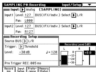
10 With the SAMPLING [REC] key still lit (on), press the SAMPLING [START/STOP] key to enter record-ready mode.
