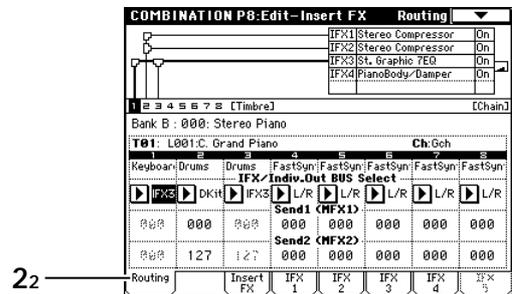
“BUS Select” (IFX/Indiv. Out BUS Select) specifies the destination to which the output of each timbre will be sent. In this combination, timbre 1 is being sent to IFX3, timbre 2 to DKit, and timbre 3 to IFX3. The LCD screen shows the effect input for each timbre. DKit means that the “BUS Select” setting specified for each key of the drum kit will apply. In this drum kit, the sound is being sent to IFX1 and 2. (PG p.170)
