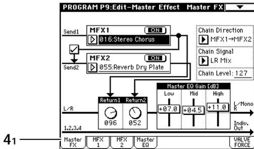
Use “MFX1” and “MFX2” to select the master effects. You can use the “Chain” check box located at the left to connect MFX1 and MFX2. “Return1” and “Return2” adjust the level that is sent from each master effect to the L/R bus.
