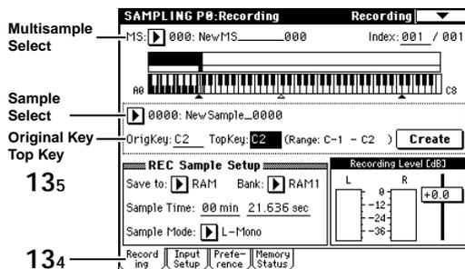
Press the Recording tab to access the P0: Recording, Recording page.
