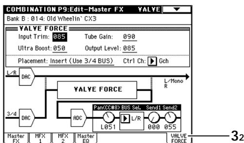
"Input Trim," "Ultra Boost," "Tube Gain," and "Output Level" adjust the sound of the Valve Force circuit. You can also set these parameters by turning the front panel VALVE FORCE knobs.
