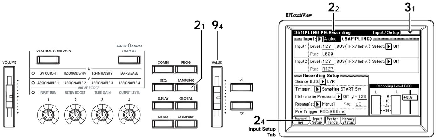
The TRITON Extreme can record mono or stereo, 48 kHz 16-bit samples. The Open Sampling System allows sampling to be performed in Sampling, Program, Combination, and Sequencer modes. (Open Sampling System) The various functions of each mode can be used while sampling.
