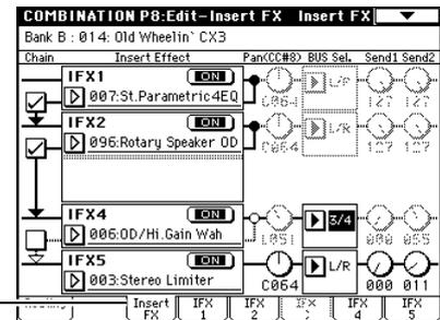
The post-IFX4 "BUS Select" is set to 3/4 (Tube). After passing through insert effect 4, the signal will be sent to Valve Force.
