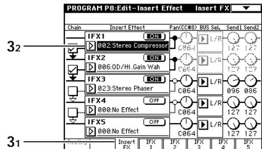
Now let's add an additional effect. Check the "Chain" check box located at the left of IFX3. This connects IFX4 to our chain of effects. Press the IFX4 OFF button to turn it ON. Then select an effect. How about 034: Stereo Auto Pan? Try selecting various effects to find the best one for your purpose.
