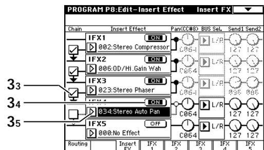
To adjust the effect depth and other effect settings, use the IFX1-IFX5 tabs to select the appropriate page, and adjust the various parameters. For details on each effect, refer to PG p.217.
